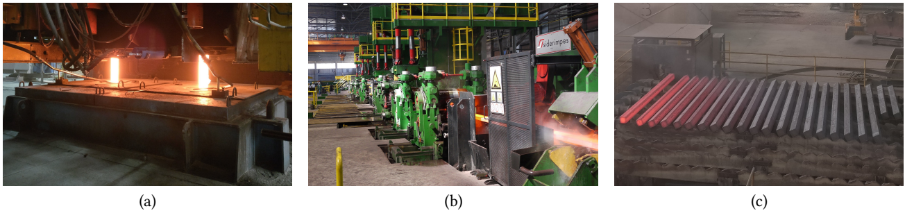
Figure 2: Continuous casting of steel: (a) pouring of molten steel into the mold where the casting process starts, (b) casting device (source: Štore Steel archive), (c) cooling of billets.
