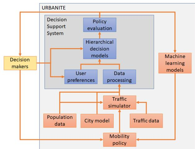
Figure 1: The architecture of the URBANITE system.
