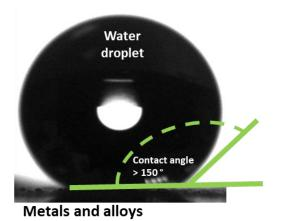
Figure 1: Water droplet on the superhydrophobic surface with contact angle above 150°
