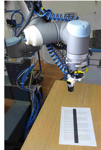
Figure 1: The robot cell composed of a UR-10 robot, a Basler acA1300-60gm area scan camera, a dedicated light source (not shown) and the dummy flat object at a calibrated distance from the robot.
