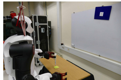
Figure 1: Writing digits with a robot using image-to-motion encoder-decoder network prediction.
