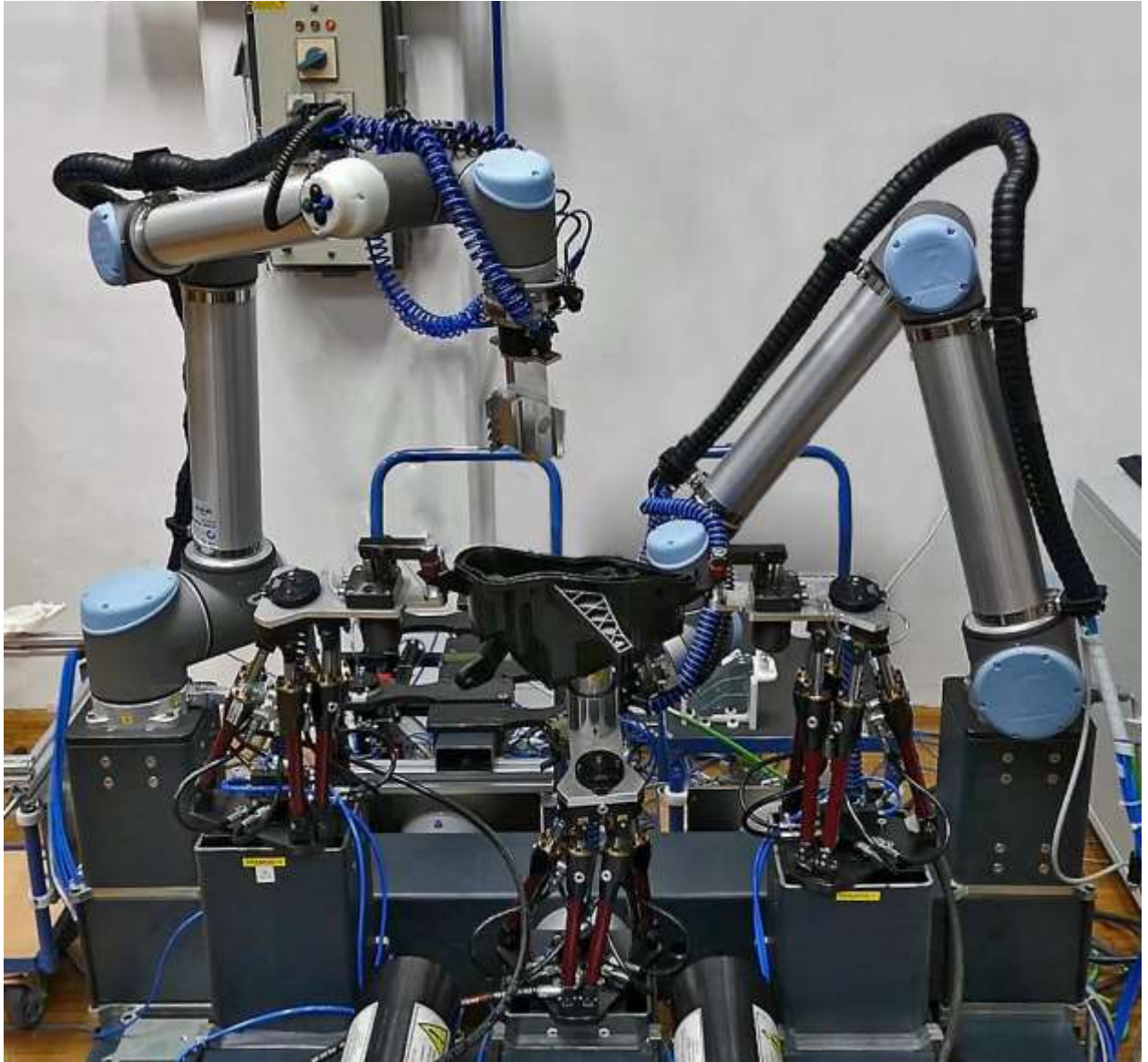
Figure 8: The reconfigurable robot cell during the assembly of an automotive headlight. Author: Timotej Gašpar, 2018.
