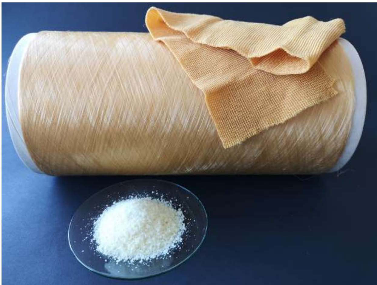
Figure 7: Flame retardant polyamide 6 copolymer and melt spun textile filament. Author: Jelena Vasiljević, 2019.
